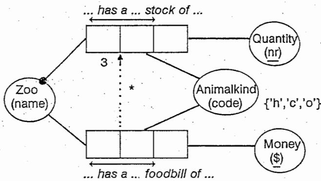
Figure 7.7 An alternative conceptual schema for the Zoo UoD
