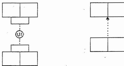
Figure 2.11 Old and new notations for a pairwise subset constraint
