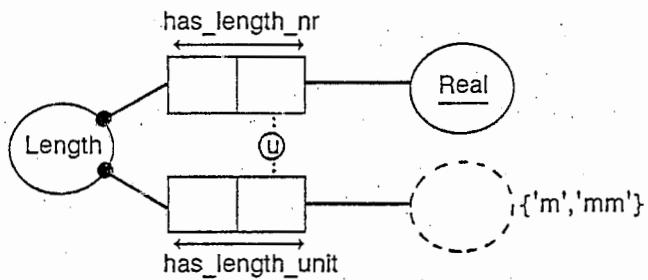
Figure 5.17 A generally inferior way to conceptualize lengths
