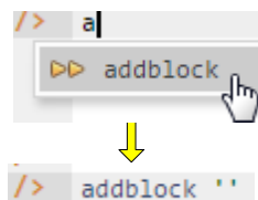
Figure 3 Invoking the addblock command in the REPL tool.
